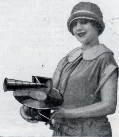
Portable Phonograph Open to Show Standard-Size Record in Place and Telescoping Horn
