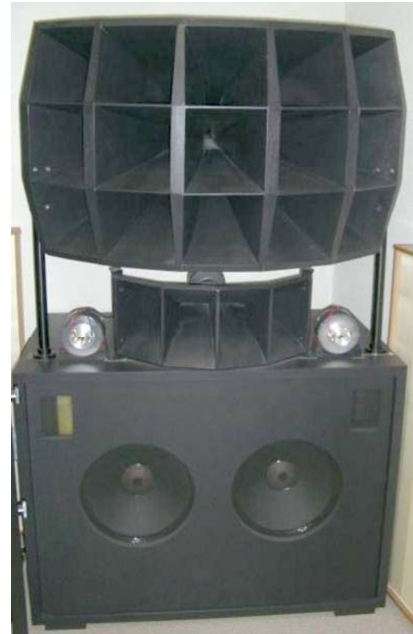
Onken 255 wood and Onken 455 wood horns on top of an Onken W bass reflex enclosure
